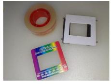
18 - Apply the diffracting grating on the slide face opposite to runners.
