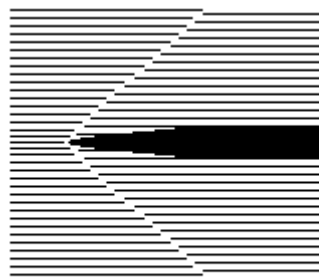
fringe jump revealing the presence of the shock wave
